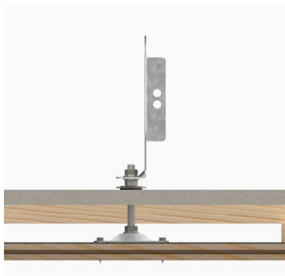
Borede hull i flate betongtakstein.
