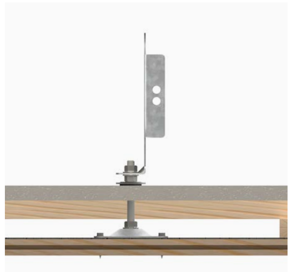
Borede hull i flate betongtakstein.
